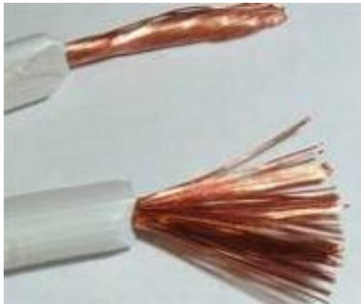
**Copper wire** is heavier, and **aluminum** is lighter and silver grey. The other main **difference between copper and aluminum wires** is the resistance of the material. ... **Copper** not only has a higher conductivity than **aluminum**, but is more ductile, with relatively high tensile strength, and **can be soldered**. Apr 12, 2010
